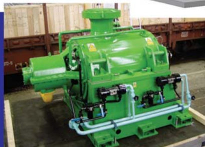
Thermal Power Plant Tušimice 8 4x200MW Feed water pump station
