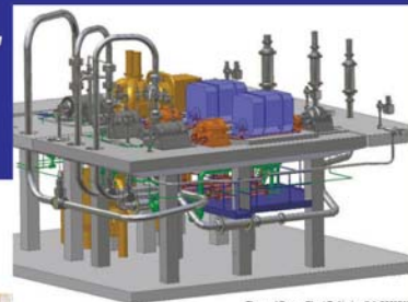
Thermal Power Plant Tušimice 8 4x200MW Feed water pump station
