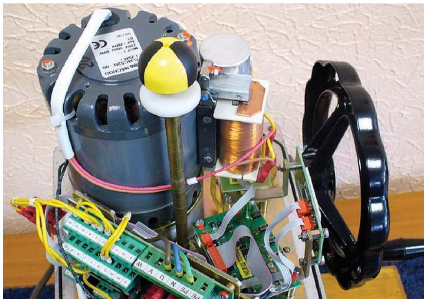
Elektronika DMS v servomotoru MOKED
