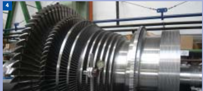
FOTO 1 – View in Machine Hall of Biomass Power Plant Sviadnov (CZ) 5,8 MWe and general view (big photo on opposite page), FOTO 2 – Wood Chips Storage and Drying in Biomass Power Plant Loučovice (CZ) 7,5 MWe, FOTO 3 – View on EPC Project Etihad Sugar Refinery (IRQ) 10 MWe, FOTO 4 – Condensing Steam Turbine 14 MW for Kazakhstan
