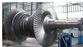
Obr. 3 NT rotor Fig. 3 Low pressure rotor
