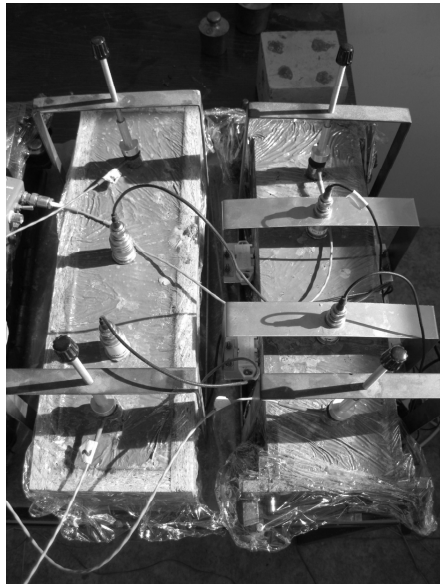
Fig. 3. Mounting acoustic emission sensors (on the left side sample from wood, on the right side sample from metal)
